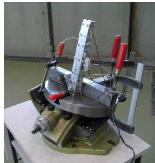
Figure 3. The inclinodeformometer on a biaxial inclinable table for calibration measurements.
