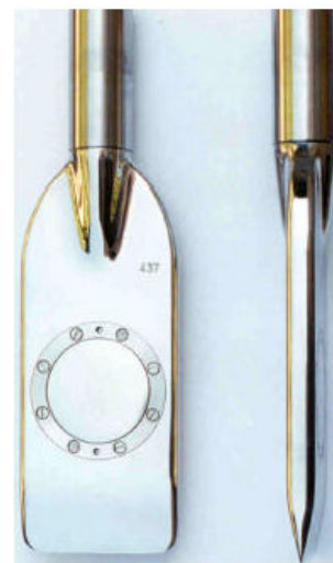
Fig. 1. The flat dilatometer - Front and side view
