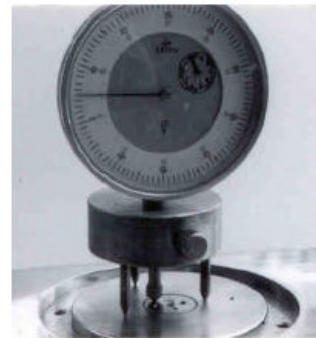
Fig. 14. "Tripod" dial gage
