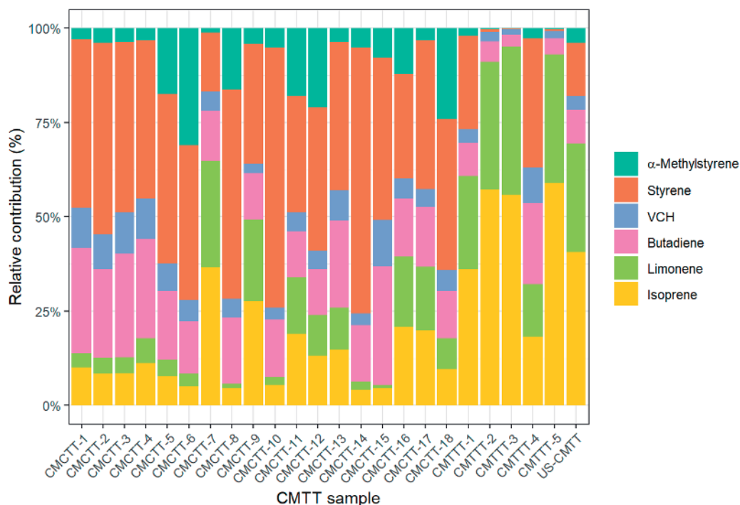
Figure 5: Relative contribution of the selected six markers (individual signal intensity relative to the sum of the intensity of all six peaks) for all cryo-milled tire tread samples. Cryo-milled tire tread (CMCTT)-1 to 18 are samples from old tires for passenger cars, and CMTT-1 to 5 are samples from old tires for trucks and buses. US-CMTT is a mixture of samples from new tires that are representative of those sold on the US market.
