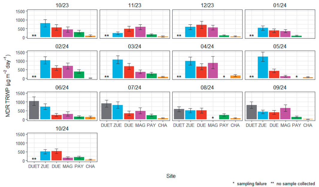
Figure 12: Mass of tire and road wear particles (TRWP) determined in dry atmospheric deposition samples collected at six sites across Switzerland from October 2023 to October 2024 (Series 1 to 14, see Annex 5.1 for exact dates). DUET: Dübendorf-Überlandstrasse, traffic; ZUE: Zurich-Kaserne, urban background; DUE Dübendorf-Empa, suburban; MAG: Magadino-Cadenazzo, rural; PAY: Payerne-MeteoSwiss, rural; CHA: Chaumont, mountainous. The title of each plot indicates the month and the year of dry deposition sampling (MM/YY), the error bars indicate the extended uncertainty for each of the analysed samples (section 3.2.4).
