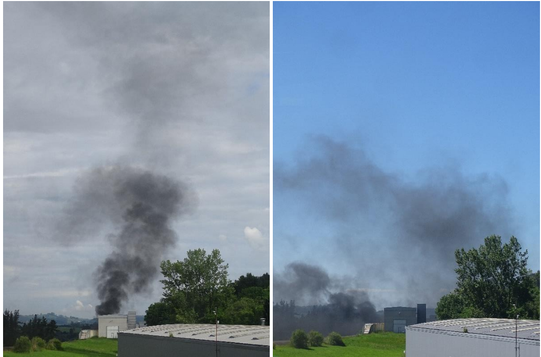
Figure 71: Smoke plume from the north portal, left: Test 1 (quiet atmosphere), right Test 3 (gusty wind)
