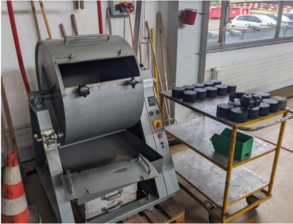
Figure 40: Los Angeles testing machine for the Cantabro test
