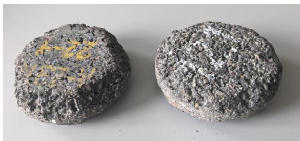
Figure 143: Cantabro test samples. Top: laboratory-prepared specimen
