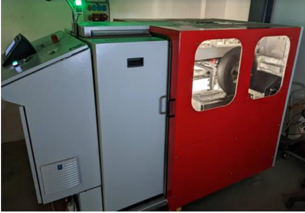
Figure 34: French Rut Tester (FRT)
