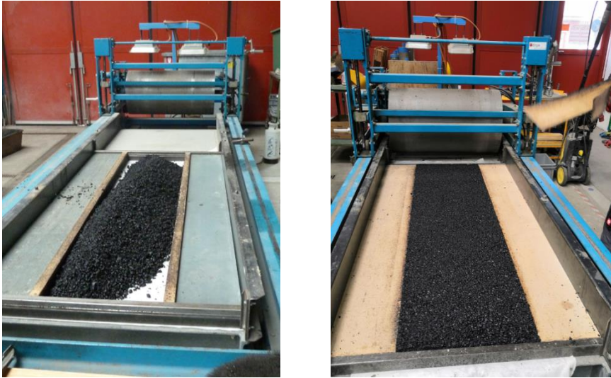
Figure 43: Roller compactor and specimen production for the MMLS3
