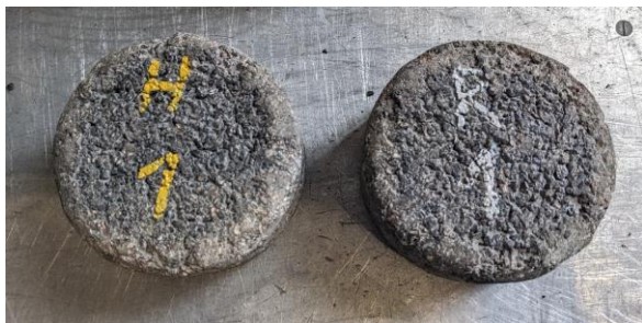
Figure 142: Cantabro test results for lab-produced SDA samples and road cores. AV is the air void content of the test samples.
