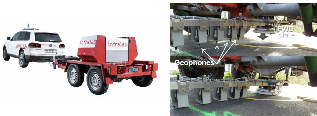
Figure 53: View of the Infralab FWD (left) and loading plate and geophones (right)
