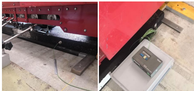
Figure 45: View of the thermocouples and data acquisition system
