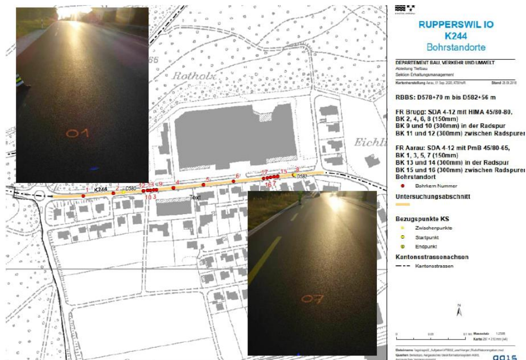
Figure 129: Location of the SDA test section in Canton AG and the location of the road cores that were taken after the construction.
