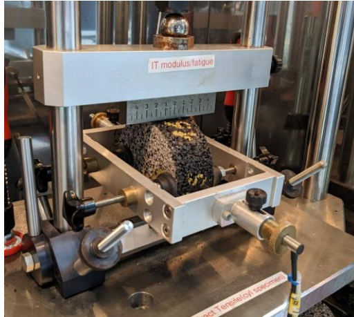
Figure 36: Stiffness modulus and fatigue test setup
