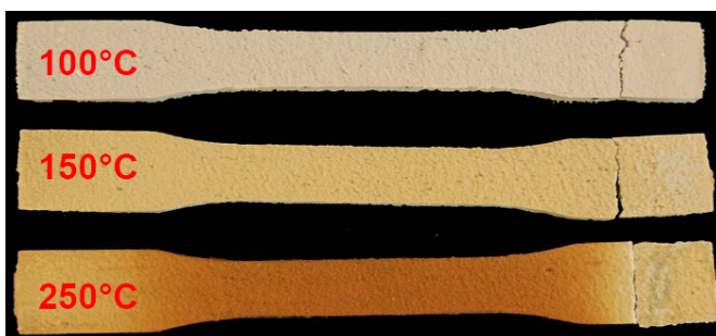
Figure 5.9 Specimen color changes and tab failure at elevated temperatures (Sikadur-30)
