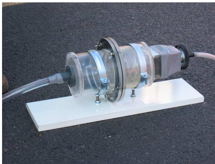
Fig. 3.11: The dust sampler. Air enters the chamber through the tube on the left. Large particles are deposited in the plexiglas tube. The particle trap is located at the right-hand side in the square block. The filter is mounted in the round, black filter holder at the right. The tube at the right connects to the pump.
