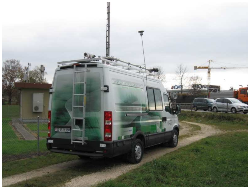
Fig. 5.4.2: PSI's mobile laboratory parked next to the NABEL station at the freeway A1 in Härkingen. The inlet for the APS is the tube with inlet head emerging from the right side window of the car.
