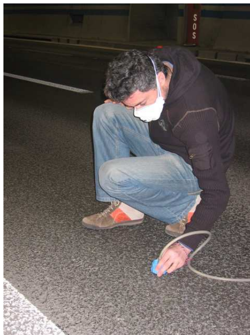
Fig. 3.13: Coarse dust sampling in the Milchbuck tunnel.
