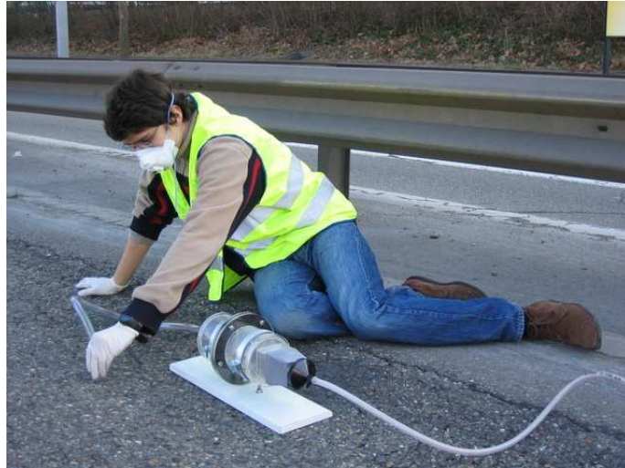
Fig. 3.12: PM10 sampling at Pfingstweidstrasse in Zürich.
