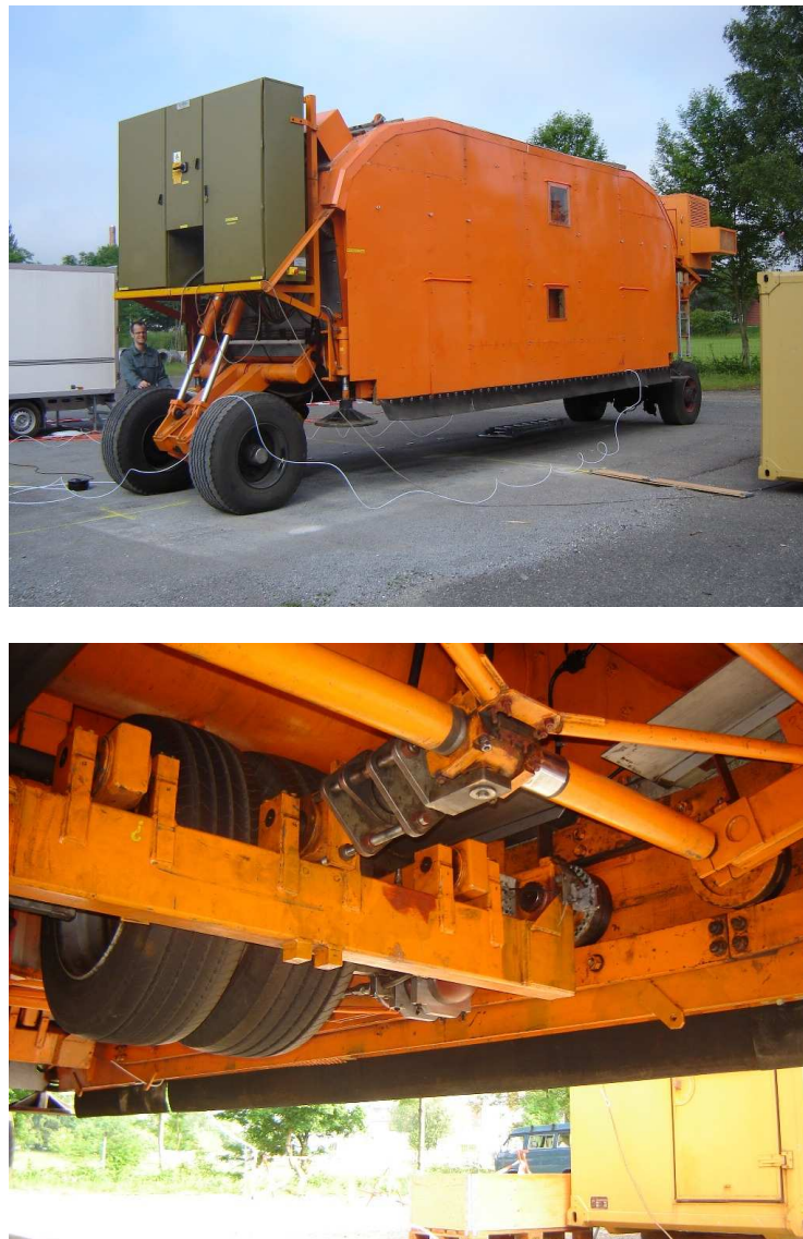
Fig. 3.8: View of the large Mobile Load Simulator (MLS, simulating the full axle load of HDV) in service position. During operation the whole device is lowered to the level of the road surface.
