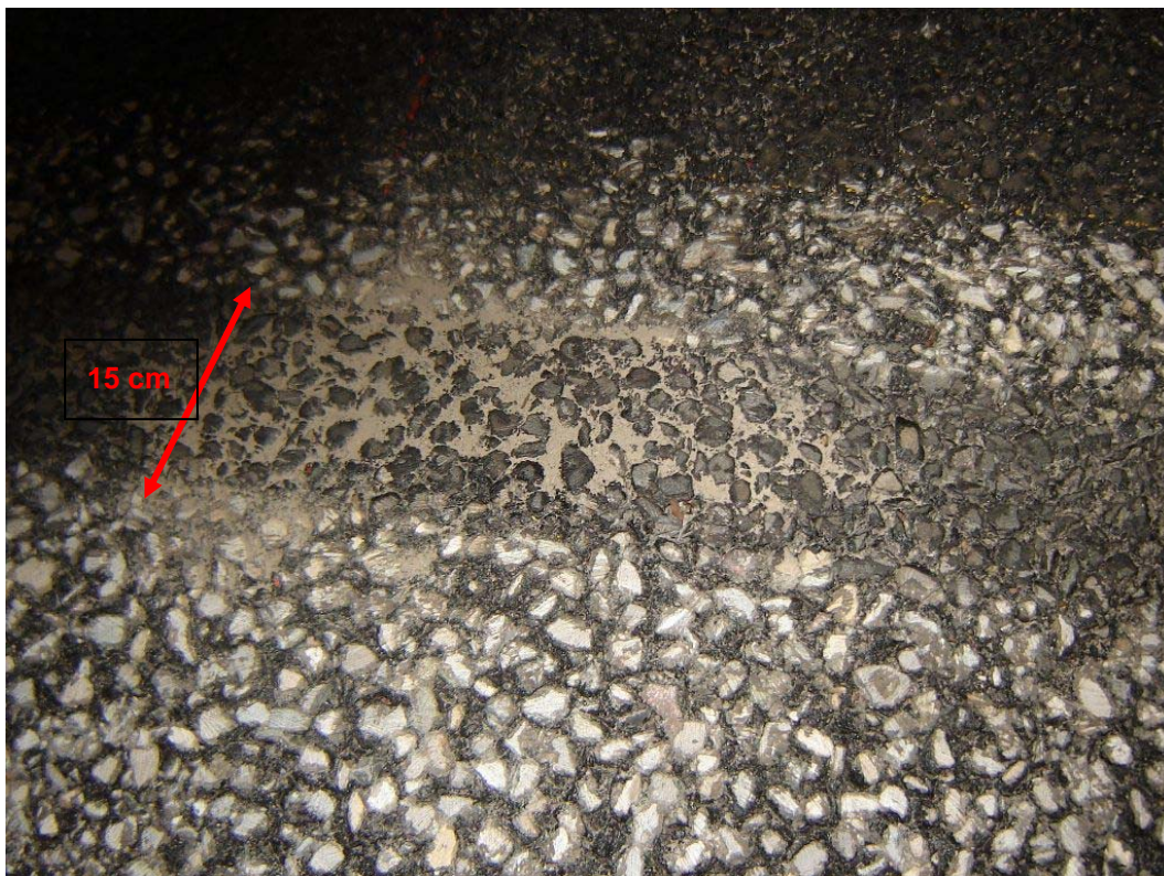
Fig. 5.2.7: View of PA pavement after resuspension experiment. Pores retaining dust are clearly visible.
