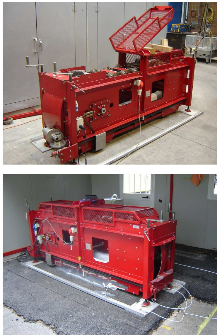
Fig. 3.7: Model Mobile Load Simulator (MMLS, simulating approx. 1/3 of the axle load of LDV): View with opened top (top) and in operation on AC pavement (bottom).
