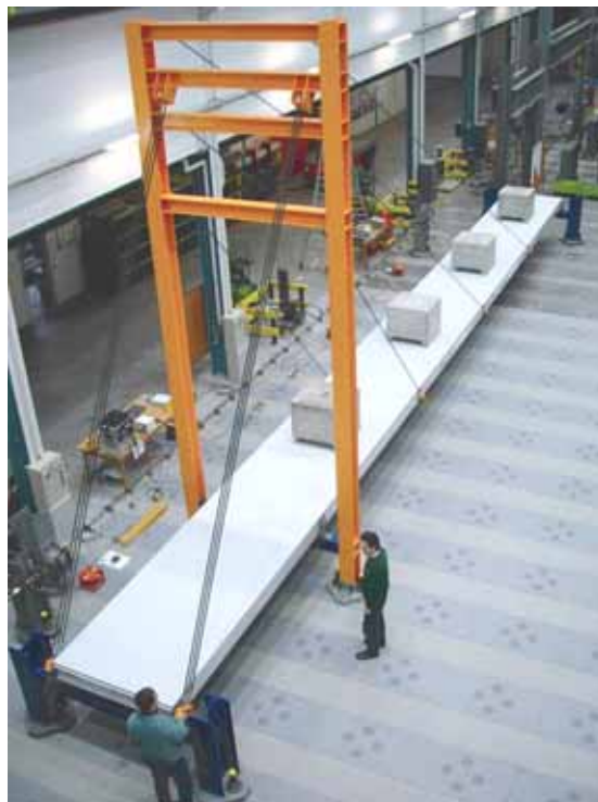
Figure 12: Full-size pedestrian cable-stayed bridge at Structural Engineering Research Laboratory, Empa.
