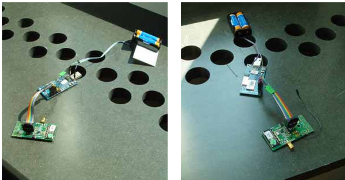
Figure 84: Some of the laboratory network nodes are in a direct sunlight (left), while the others are in the shadow (right).
