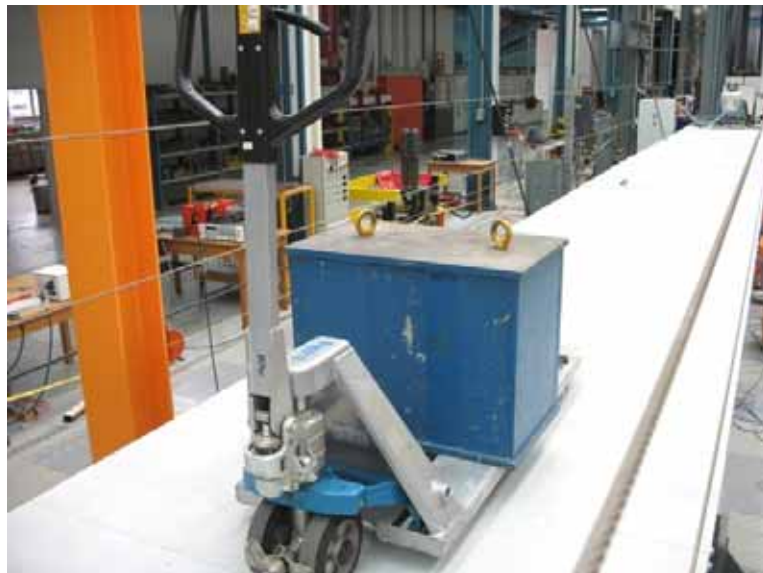
Figure 48: A mass of about 500kg was moved across the bridge deck in order to observe the changes in cable natural frequencies.
