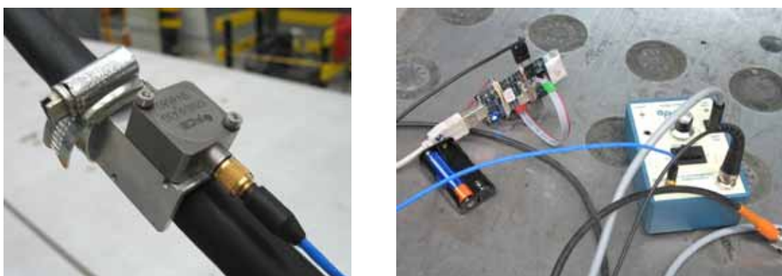
Figure 45: (left) A precision acceleration sensor mounted on a cable stay of the lab bridge. (right) Dedicated sensor signal amplifier.
