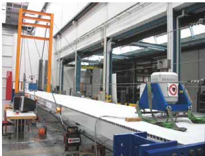
Figure 46: A shaker producing broad band random vibrations was used to excite the cable stays.
