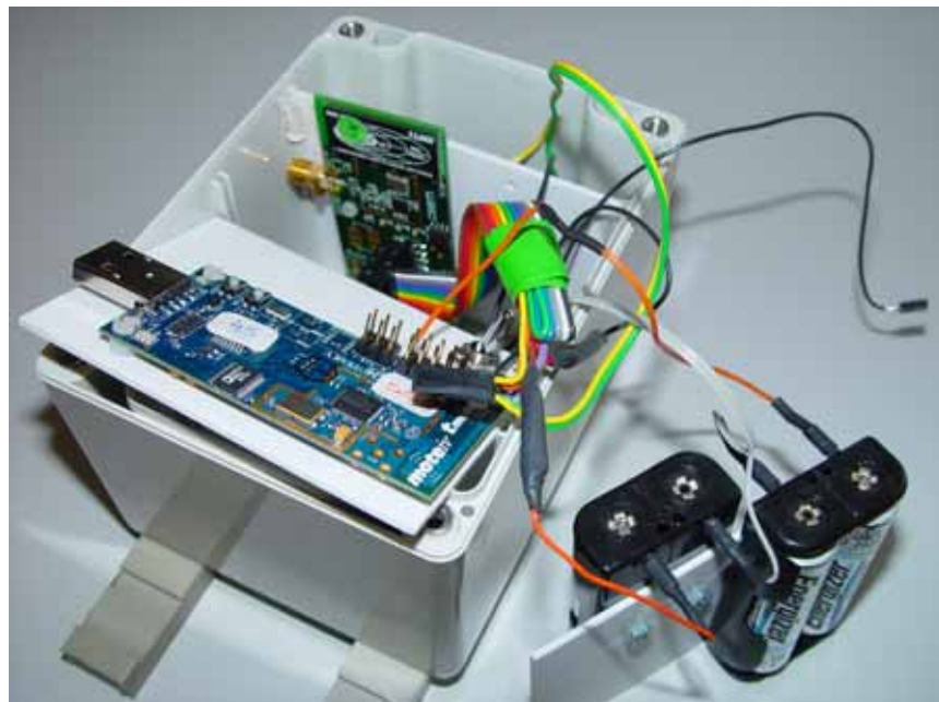
Figure 63: Hardware components were mounted on the plastic boards which were inserted into the mounting rails of the enclosure.
