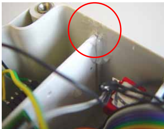
Figure 64: Board holding the sensor module is glued to the housing.
