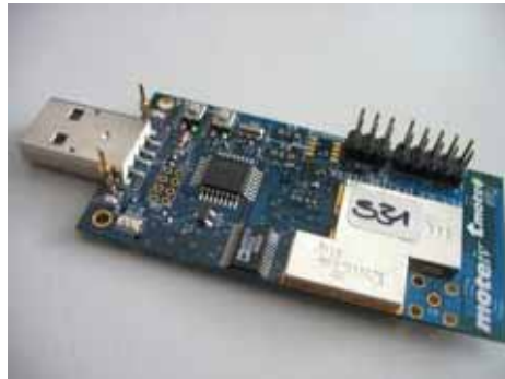
Figure 15: Tmote Sky platform was chosen as the application board.
