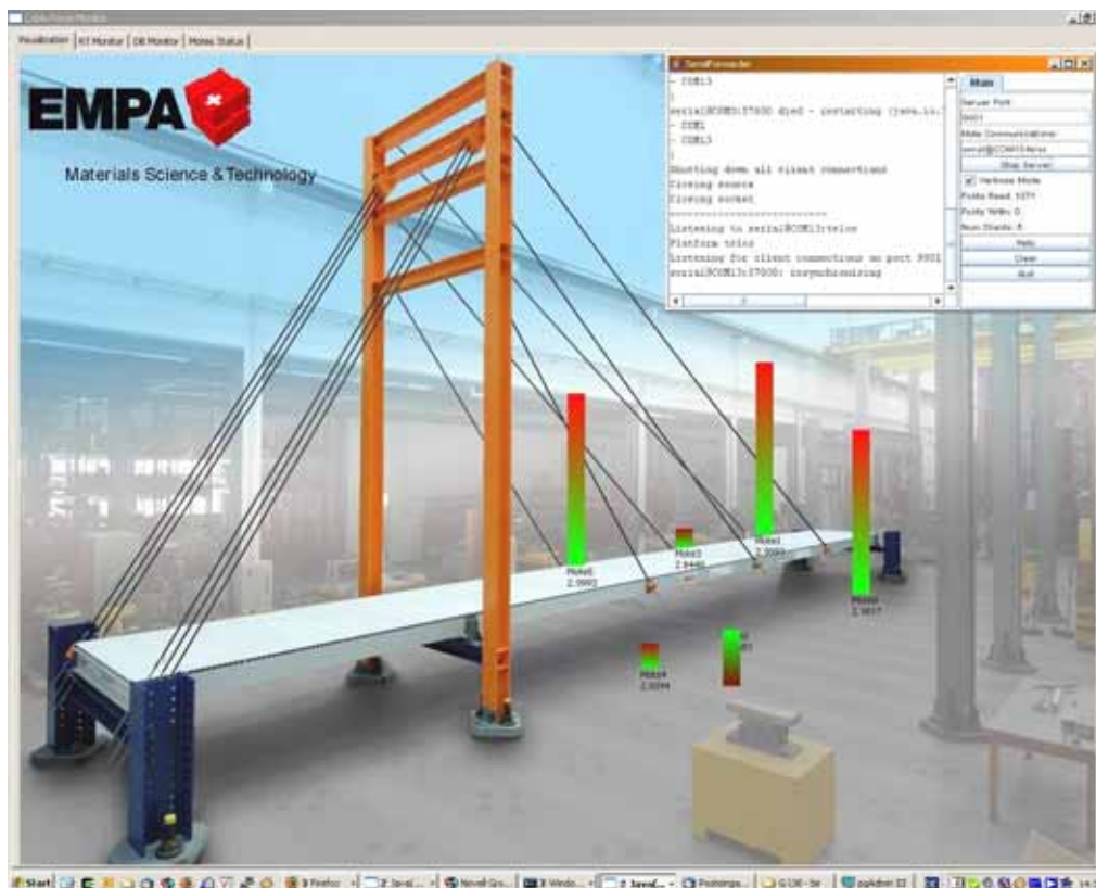
Figure 55: Visualisation of changes in cable tension force (natural frequencies).
