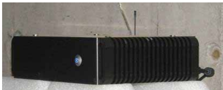
Figure 20: Base-station is an industrial embedded PC with a wireless Internet connection.
