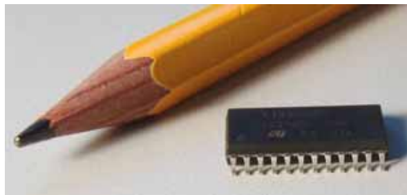
Figure 18: LIS3L02 MEMS accelerometer from ST Microelectronics.
