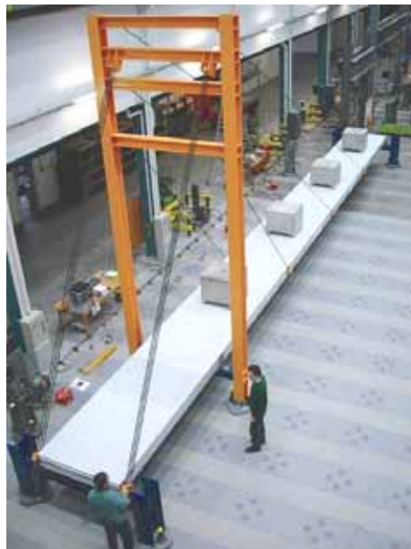
Figure 43: Full-scale pedestrian bridge where the WSN system was verified in a short-term demonstration test at the Structural Engineering Research Laboratory at Empa.
