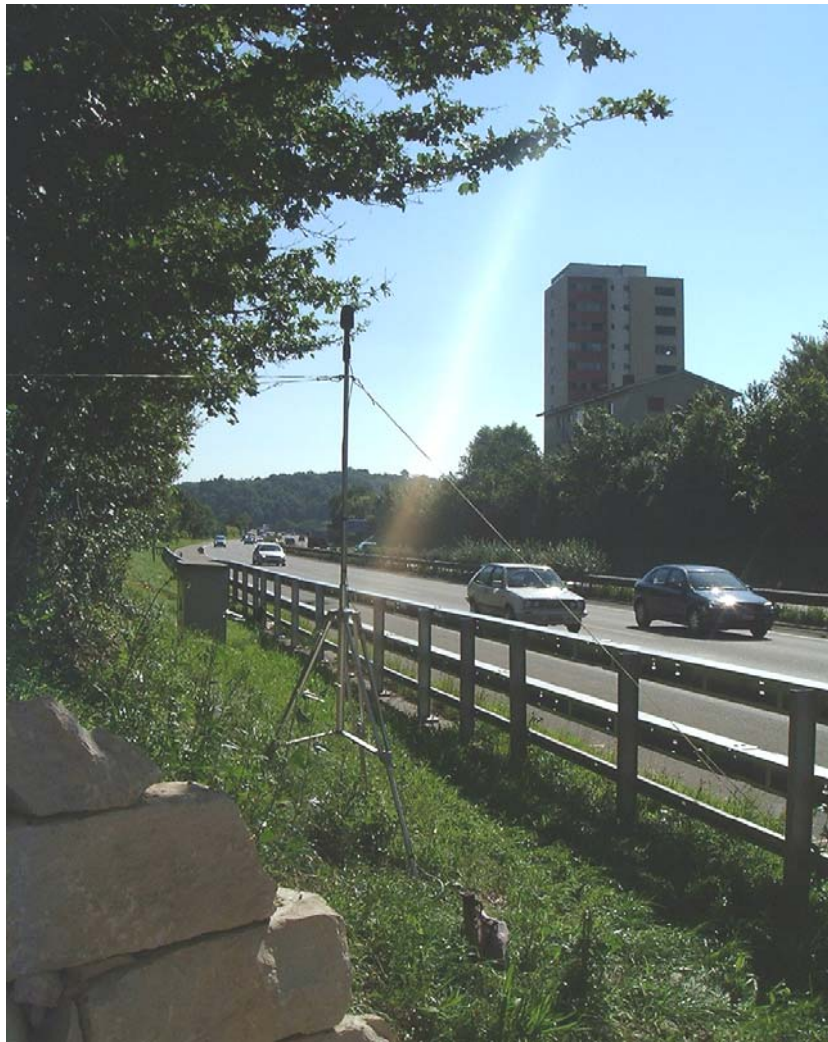
Figure 10. 7: Measurement location Lenzburg showing the microphone position 3 m above road level
