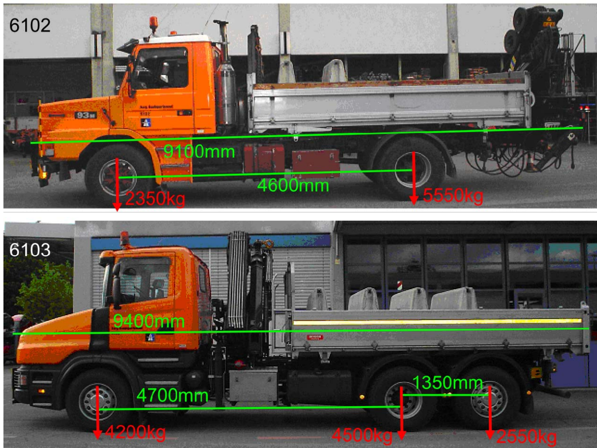
Figure 17. 2: Vehicles used in the finite element model validation with the lengths and wheel loads shown
