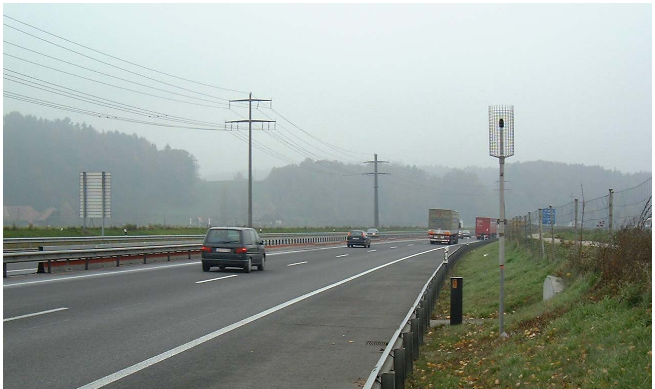
Figure 10. 2: Measurement location Reiden. The microphone is protected with a grid basket
