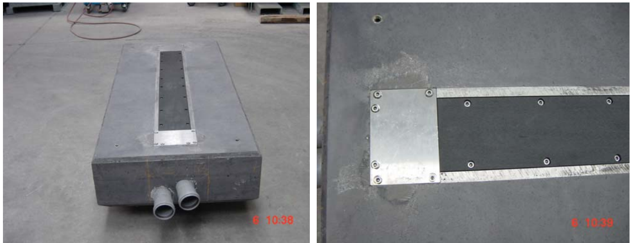
Figure 6. 13: Modulas replacement “Dummy” placed in the concrete element
