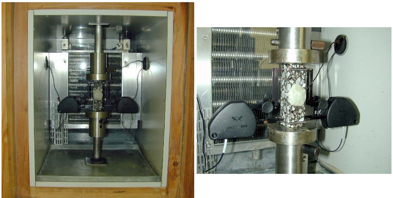
Figure 9. 14: Assembly of the sample in the conditioning chamber at LAVOC for the direct tension test
