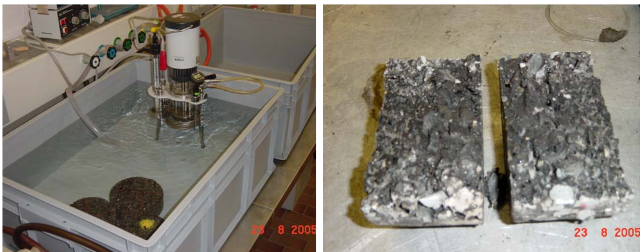
Figure 10. 29 : Conditioning of the specimen in a water bath (left) and fracture surface of the twinlay after ITS test at 5°C.
