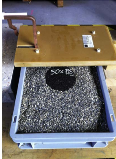
Fig. 6.1 Sample in a sandbox for induction healing.
