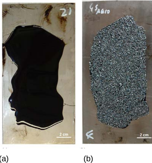
Fig. 5.6 (a) Steel plate with virgin bitumen 70/100 pen (b) Steel plate with virgin bitumen 70/100 pen and cast iron particles.
