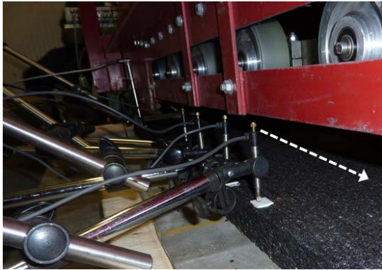
Fig. 6.14 Detail of the vertical deformation sensors.
