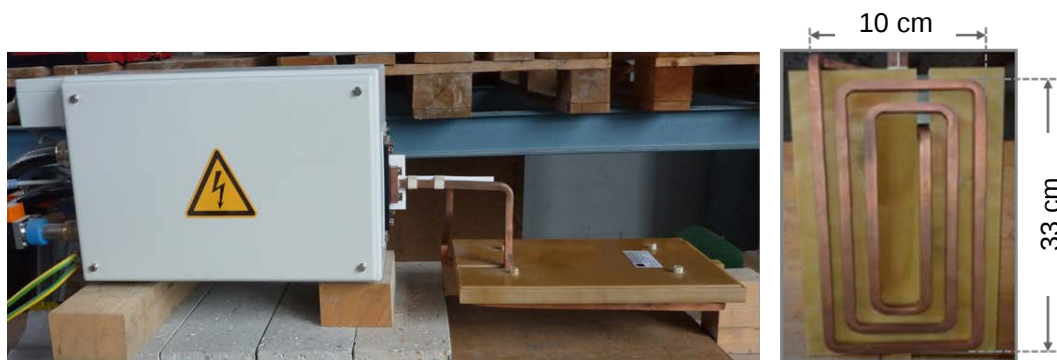
Fig. 3.23 Induction heating source with matching box and coil inductor (left) and detail of shape of the coil inductor (right).
