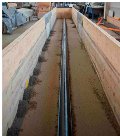
Figure 6-21: Embedment of the instrumented tube into the test setup.
