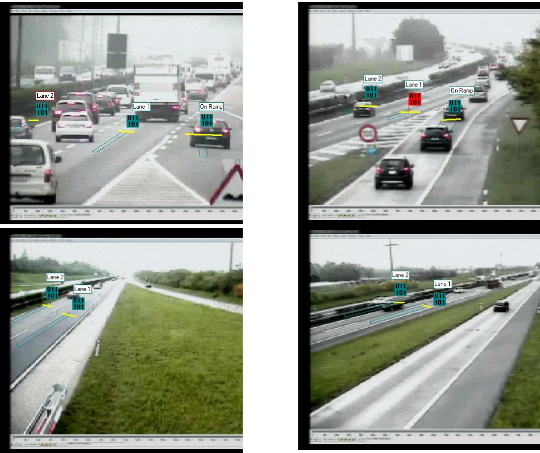
Figure 3 Snapshots of processed video data collection with Autoscope
