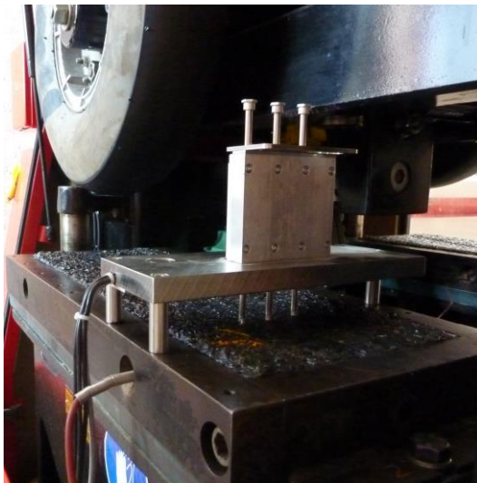
Figure 5. 17 Measurement of permanent deformation of the specimen
