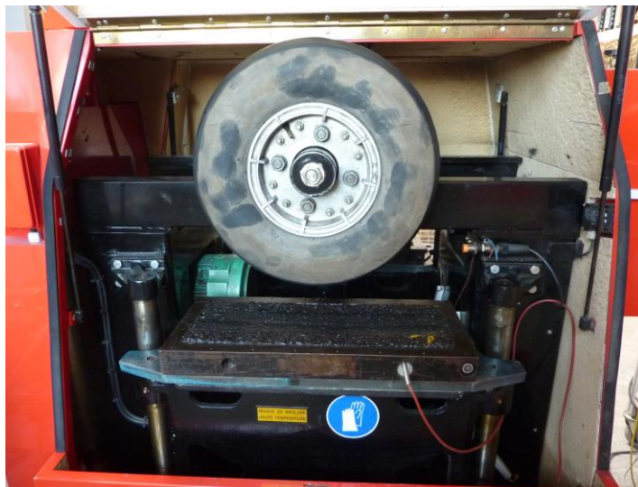
Figure 5. 15 Specimen in the French wheel tracking device
