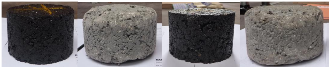
Figure 5. 20 Mx05, AC 11 S with 0%RAP before and after PL Tests, left and Mx 07, AC 11 S with 40%RAP before and after PL Tests, right
