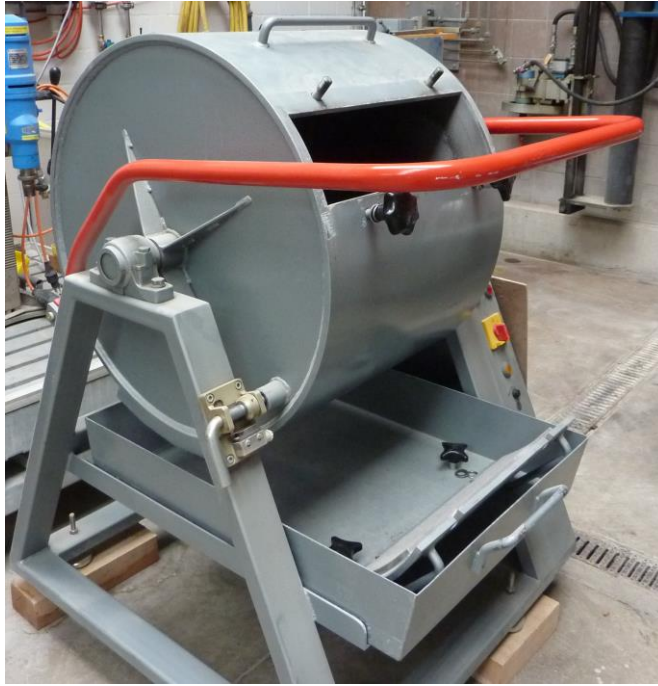
Figure 5. 19 Los Angeles drum used for the particle loss tests at Empa
