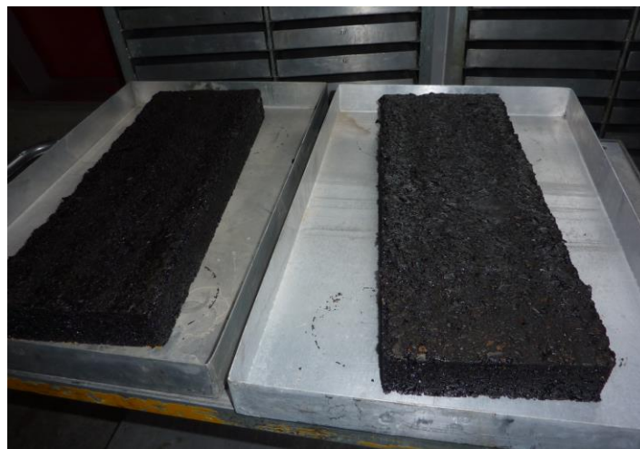
Figure 4. 2. Long Term Oven Aging (LTOA) of wheel tracking specimens in a forced draft oven
