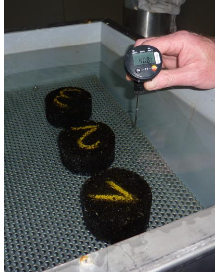
Figure 3. 1 Water conditioning of specimen at 40°C
