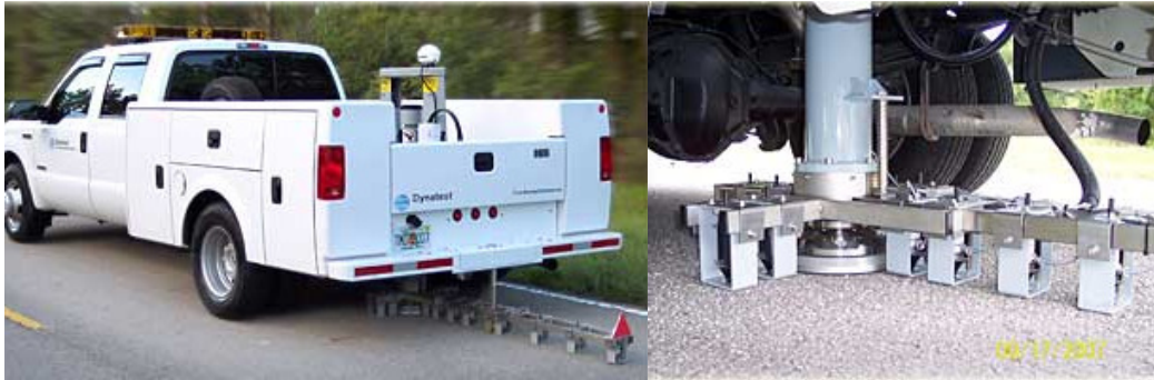
Abb. 3.2 Falling Weight Deflectometer (Dynatest)
