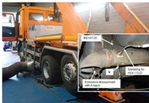
Tested vehicle and measuring apparatus on the LARAG HD chassis dyno
