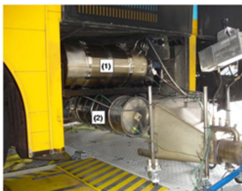
Fig.3a: Retrofitted combined System. DPF (1) & SCR (2)
