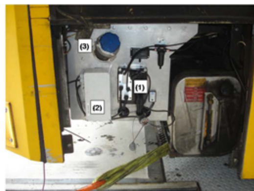
Fig.3b: Urea Dosing System UDS (1), datalogger (2) & Adblue tank (3)
