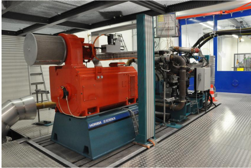
Figure 7. 1 Heavy duty engine test bench at Empa showing the dynamometer on the left side and the engine on the right side
