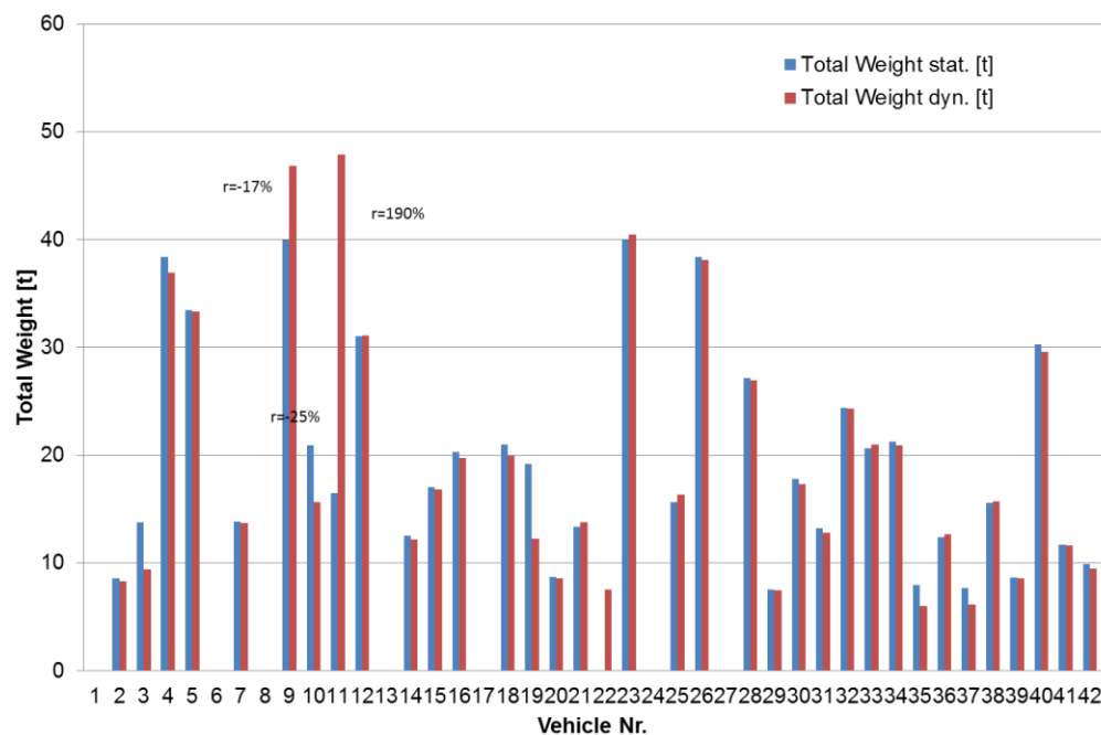
Figure 9. 2 Total vehicle mass of the 42 vehicles investigated shows that 93% of the measurements were within 7% tolerance
